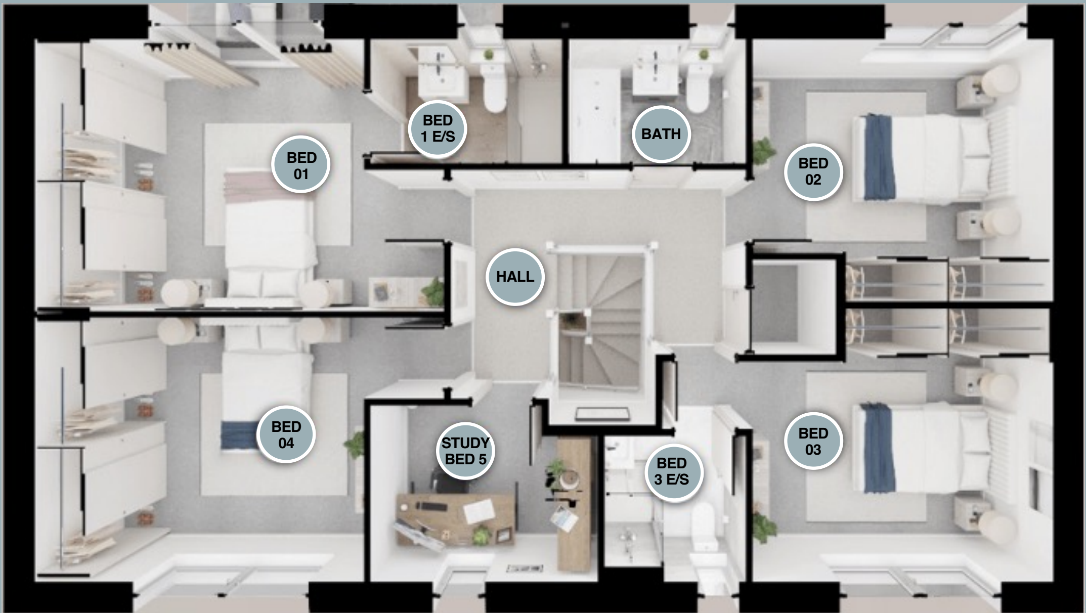
FIRST FLOOR PLAN – PLOTS 1, 3 & 4. Gross Internal First Floor 104.4 sq.m. TOTAL GROSS 220.3 sq.m.
